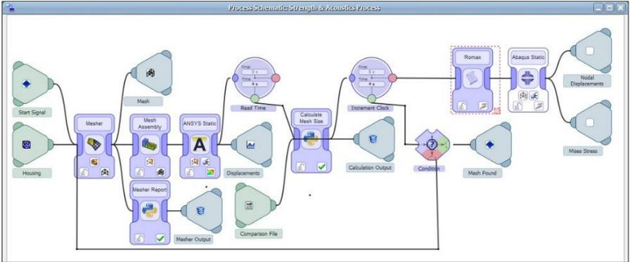
With Aras Simulation Management, you can capture, enforce, and scale simulation best practices to more enterprise teams, automatically generating model files and chaining together multiphysics simulation tools.
