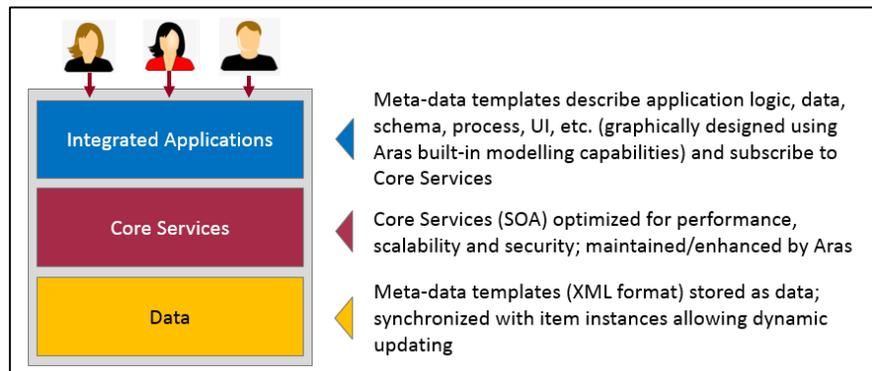
For those architects looking for a generic description, Aras Innovator is a Web-based, n-tier, service-oriented architecture composed of web clients, application server(s), database(s) and file server(s) and is based entirely on standard Internet protocols including HTTP / HTTPS, XML and SOAP (Simple Object Access Protocol).
