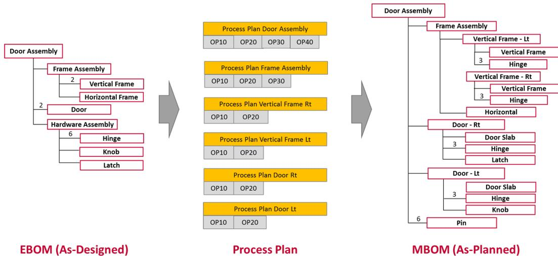
Figure 1—EBOM and MBOM for a Door Assembly
